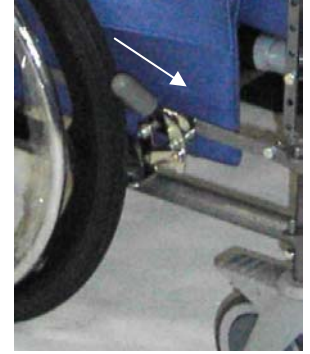
Wheel lock in unlocked position. (Pull toward front of chair to lock)
